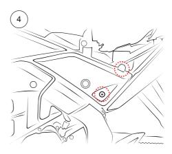
Take off the LH lateral fearing by removing 2 screws on the top and 4 screws on the bottom.
