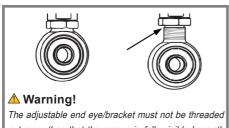
out more than that the groove is fully visible beneath the lock nut. This is maximum length. After adjusting, make sure that the lock nut is tightened (40Nm).
