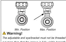
The adjustable end eye/bracket must not be threaded out more than that the groove is fully visible beneath the lock nut. This is maximum length. After adjusting, make sure that the lock nut is tightened (30Nm).
