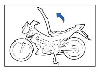
Remove the fairing by loosening the screws on both sides (1)(2).
