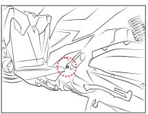
8-4 Remove 2 screws (left and right),under the rear light and unplug the rear light wiring.
