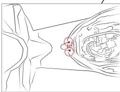
8-3 Remove 2 screws (left and right),(under the fearing)
