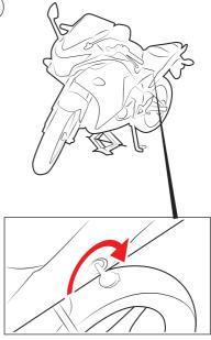
Remove the driver seat by loosening the two screws.
