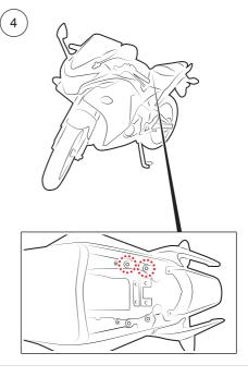
Remove the seat cowl by loosening the two screws.
