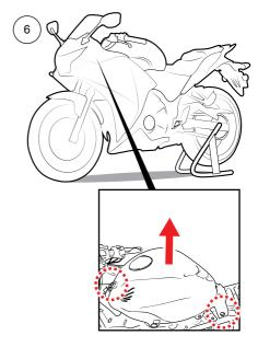
Loosen four (4) bolts of airbox with 10 mm socket in order to have more space when remove upper shock absorber mounting point.
